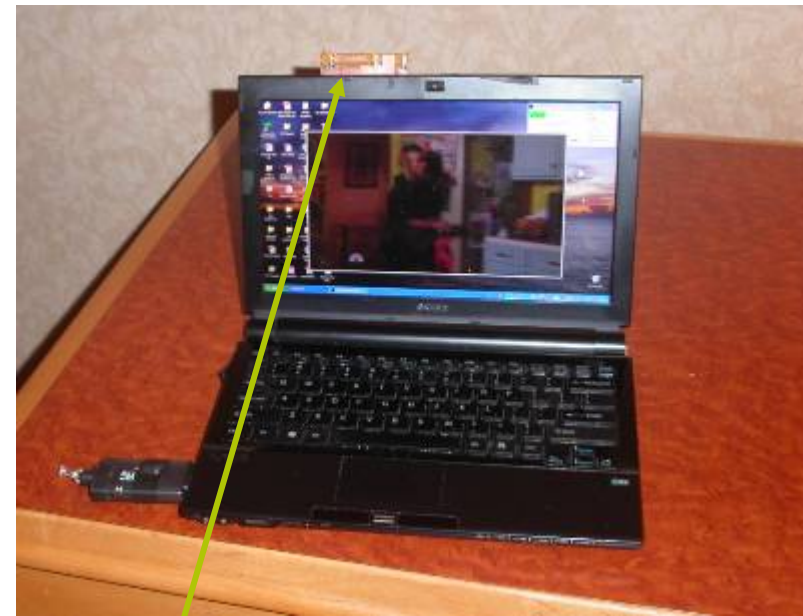
Antenna pcb taped behind to lid of laptop
