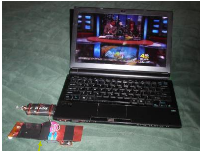
Antenna on pcb lying in front of 11-in laptop
