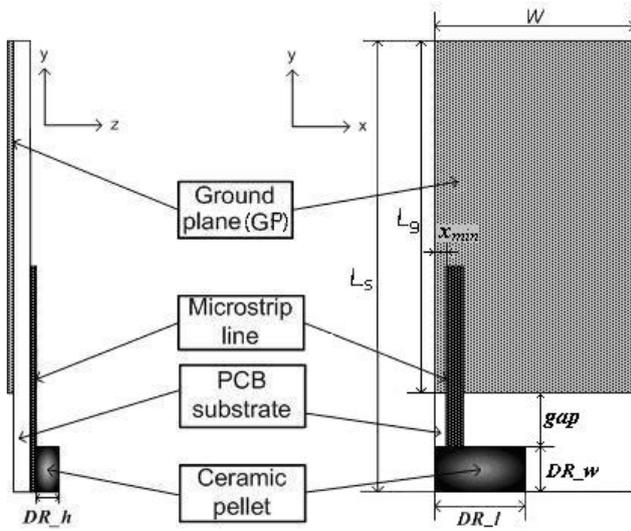
Fig. 1. Geometry of the prototype antenna
