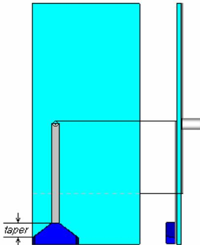
Fig. 4. Geometry of the trapezoidal pellet antenna
