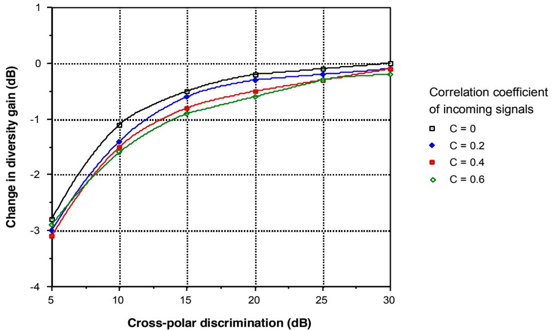
Figure 5: Reduction in diversity gain as a function of antenna XPD and the correlation of the incoming orthogonal signal components.
