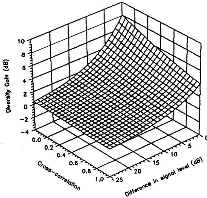
Diversity gain at 90% signal reliability as a function of cross- correlation and mean branch signal level difference. (Maximal ratio combining)
