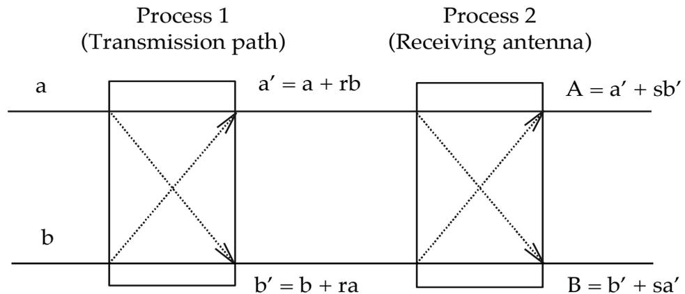
Figure 1: Mixing process 1 is used to create two signal branches with the required correlation. Process 2 represents the imperfect cross-polar discrimination of the receiving antenna.
