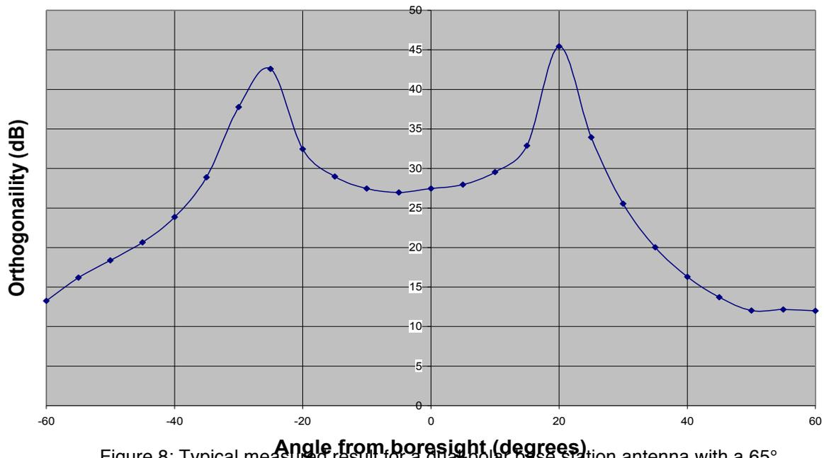
Figure 8: Typical measured result for a dual-polar base station antenna with a  $65^\circ$  azimuth 3-dB beamwidth
