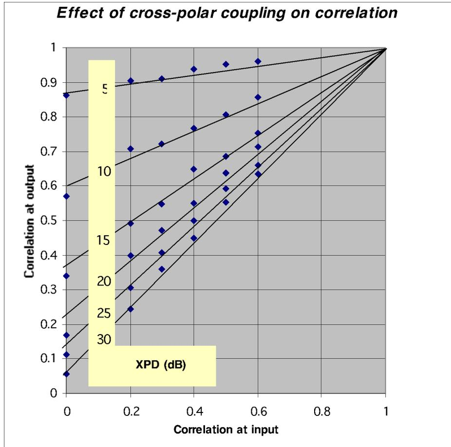
Figure 2: Correlation of incoming signals and resulting output from a dual polar antenna with finite cross-polar discrimination.
